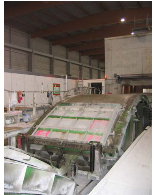
fig 4. tunnel lining segment production at Glass GmbH
